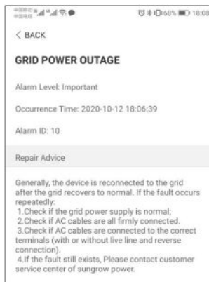
figure 7-9 Detailed Fault Alarm Information
