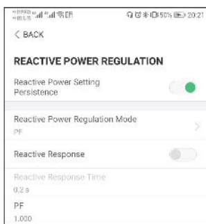
figure 7-17 Reactive Power Regulation
